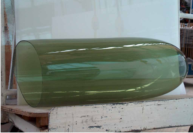
FIG. 5.5 Cylinder glass was another common glass types until 19 th century / Photo: RCE
