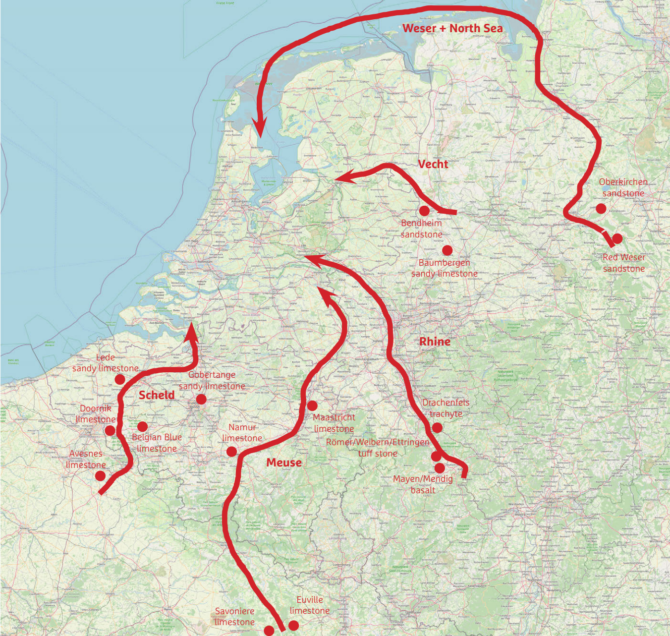
FIG. 2.2 Areas of origin of natural stone types used in historic buildings in the Netherlands with their direction of distribution (base map: openstreetmap)
