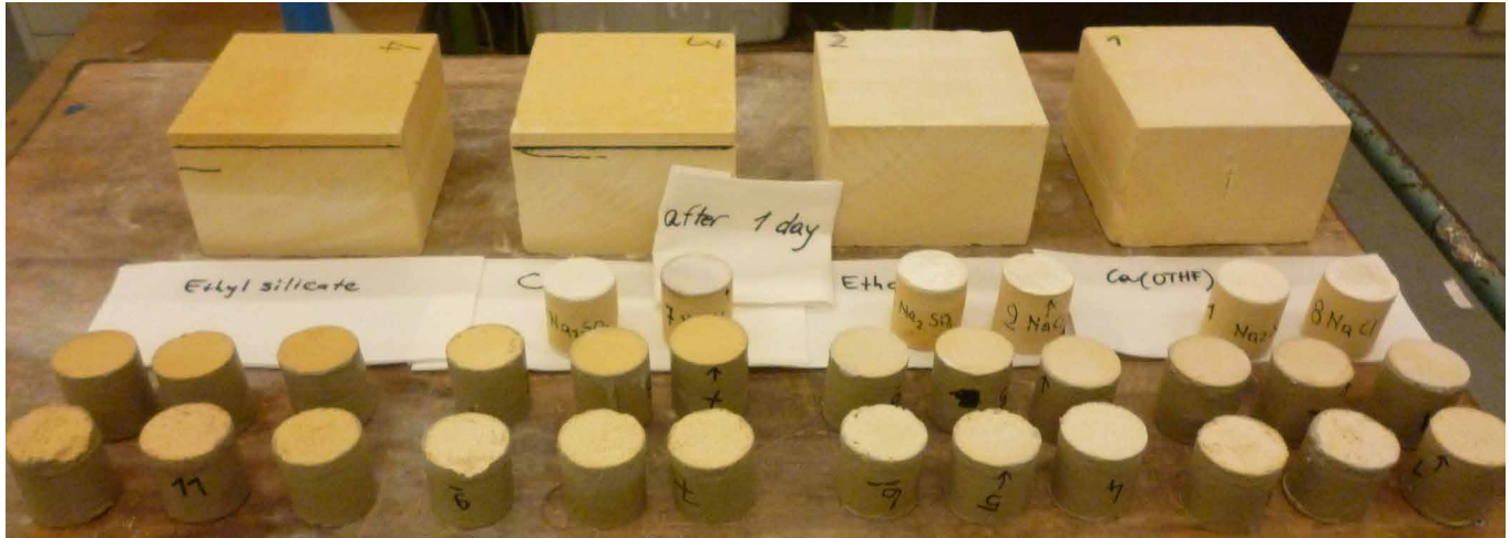
FIG. 4.23 Maastricht limestone 1 day after the application of different consolidation products: product 2 and to a lesser degree product 1, have caused whitening of the surface / Photo: B. Lubelli
