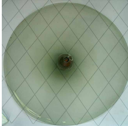
FIG. 5.3 The term 'bull's eye' refers to the thicker centre area of crown glass around the pontil mark / Photo: RCE
