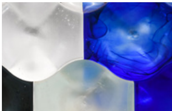
Osteomorphic: Interlocking system out of recycled window panes, crystalware, artware, CRT screens and optical lenses.
