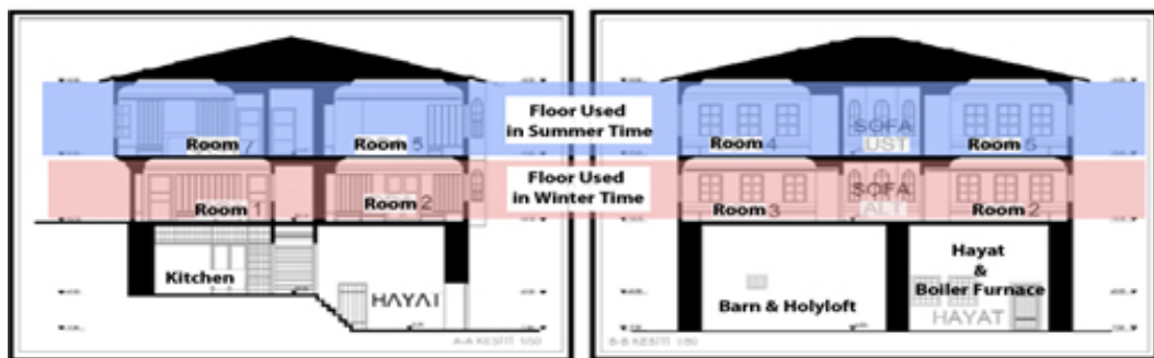
FIG. 10 Sections of Haci Huseyinler house and winter and summer time's parts. Sections of Haci Huseyinler house and winter and summer time's parts
