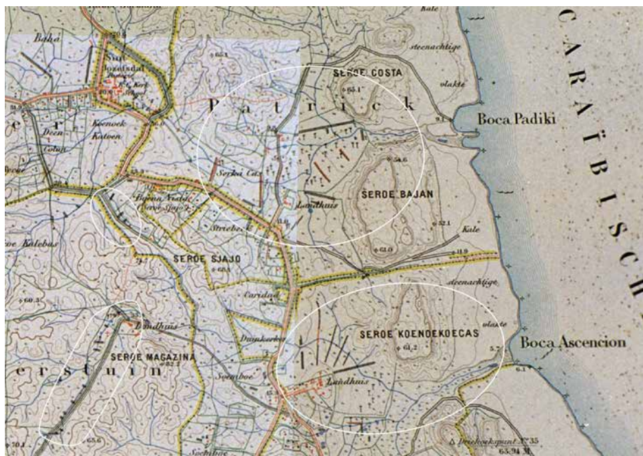
FIG. 10 The detail of map C.05 shows the large dam system near the manor houses with waterplantages North-east of Willemstad with rooien leading to water reservoirs on the sandy boca (outlets) to the sea. The small dam systems are located on the higher sloped terrain west of the manor houses where possibly the kostgrondjes of the Afrocan Caribbean small holder farmers. Maker: Werbata-Jonckheer. Source: authors own.
