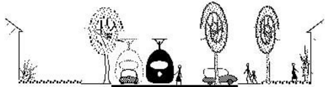
30km/h PUBLIC AREA: Cross-section based on frequent crossing by pedestrians and cyclists at points designed for the purpose rails set into the surface
