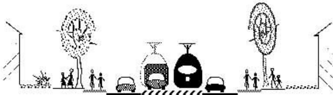
50km/h PARALLEL WITH LOCAL ACCESS ROAD: Cross-section based on dedicated lane for tram – possibly also for use by services, taxi and in emergencies – marked out by differences in height with lanes for other traffic: FENCES at dangerous places and where numbers of pedestrians crossing the track would be too high; priority at busy intersections
