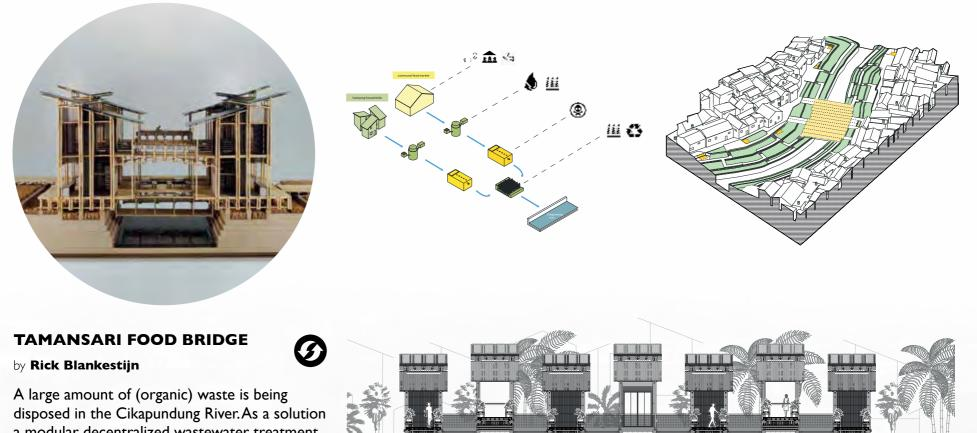
a modular decentralized wastewater treatment system has been developed which integrates different public functions. Finally the Tamansari Food Bridge has been designed, which enables kampung dwellers to cross the river and benefit from the produced fertilizers and biogas by growing and selling food.
