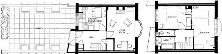
Plan views of a maisonette over a shop, showing lower and upper floors
