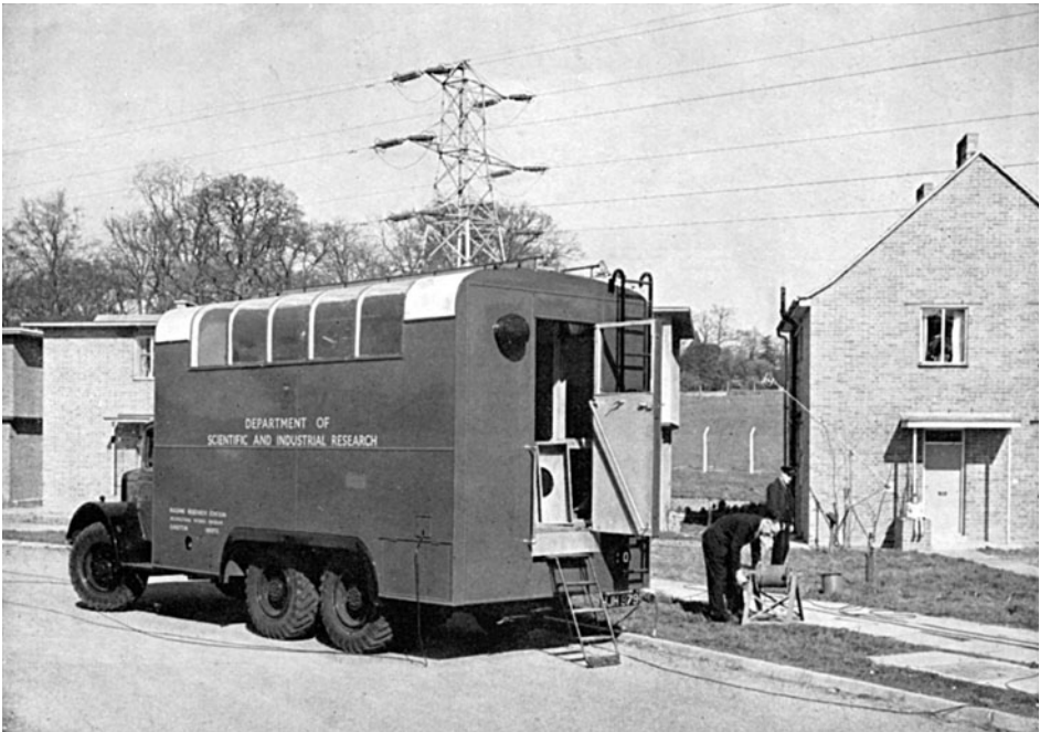
The Mobile Acoustics Laboratory for measuring sound insulation. It was used in the Royal Festival Hall
