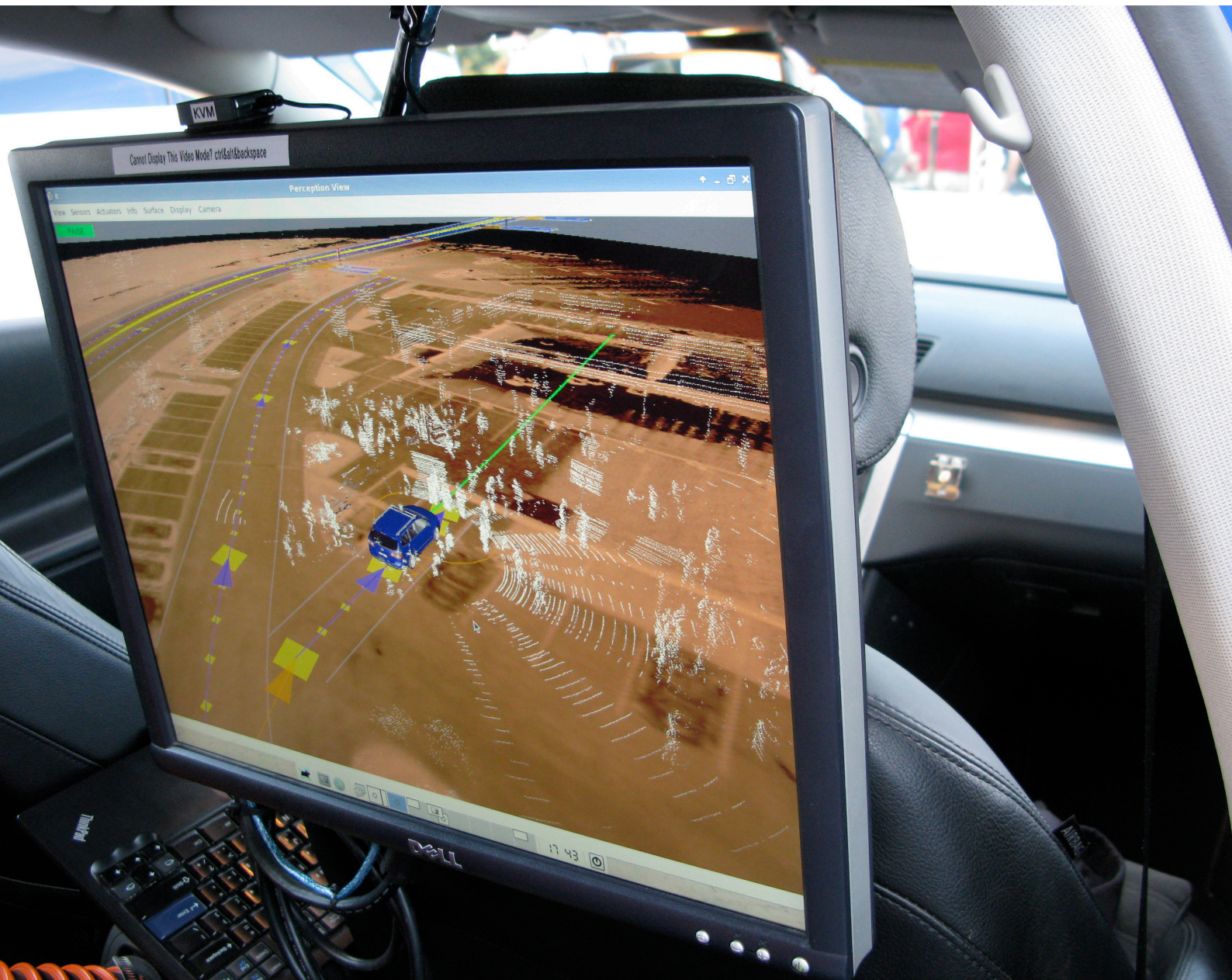
Fig.1 LIDAR rendering in real-time a 3D image of the environment around a car. Photo in an automated car by Steve Jurvetson.
