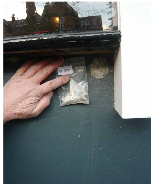
FIG. 3.19 Plaster sample from the wall below the studio window on Prins Hendriklaan
