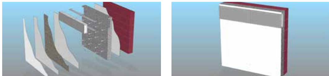
FIG. 1 Scheme of a ventilated façade
