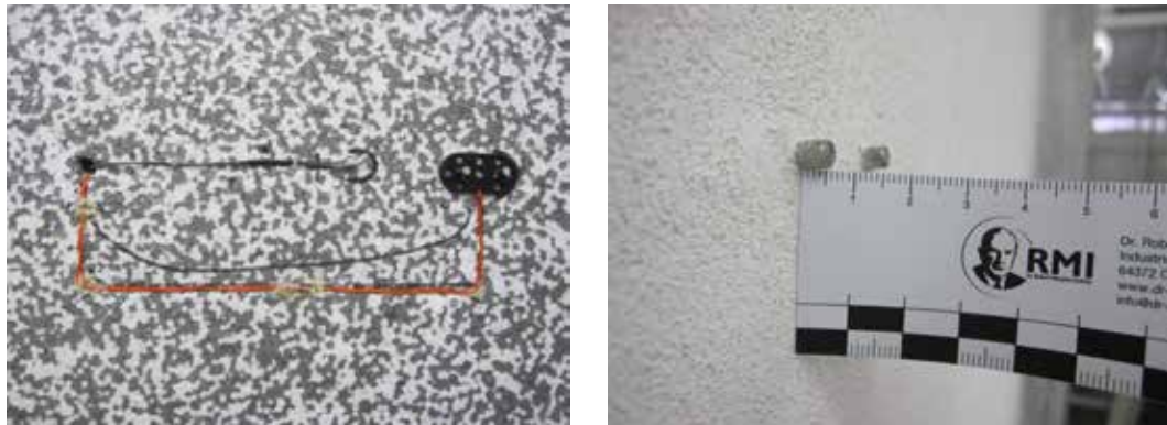
FIG. 2 Left image: Temperature sensor (left) and humidity sensor (right) attached to EPS as thermal insulation material; right image: sensor pins of humidity sensor after application of the top coat
