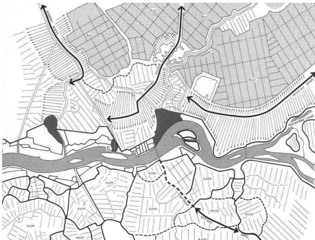
FIGURE 3.3 The spatial structure of Rotterdam: north of the river, it is defined by long lines of dikes and quays, and south of the river it is dominated by ring polders. Source: Palmboom (1987)
