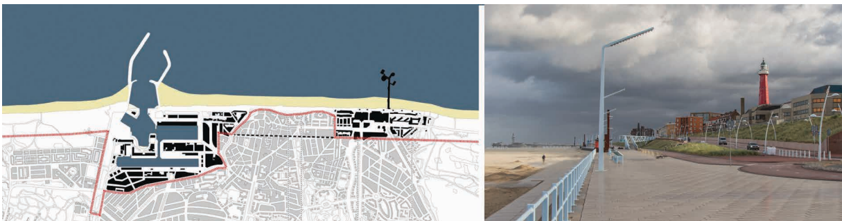
FIGURE 8.19 (left) The water defence line that runs through the urbanized seafront of Scheveningen. In the middle part the water defence line has already been brought seaward, during a recent reinforcement. The landscape design was created by De Solà-Morales (photo on the right: Rijkswaterstaat, Harry van Reeken).
