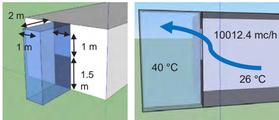
Need air flow rate/floor:  $10800 \text{ m}^3/\text{h}$
