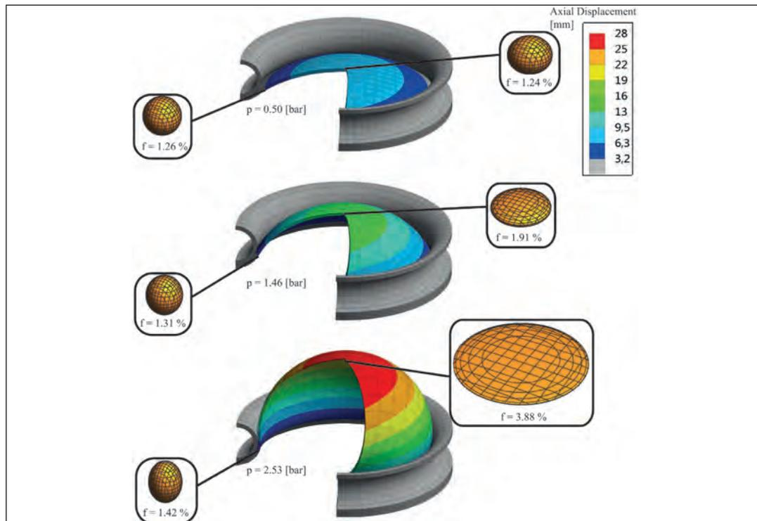
Fig. 1. Material modelling of the structural silicone connections
