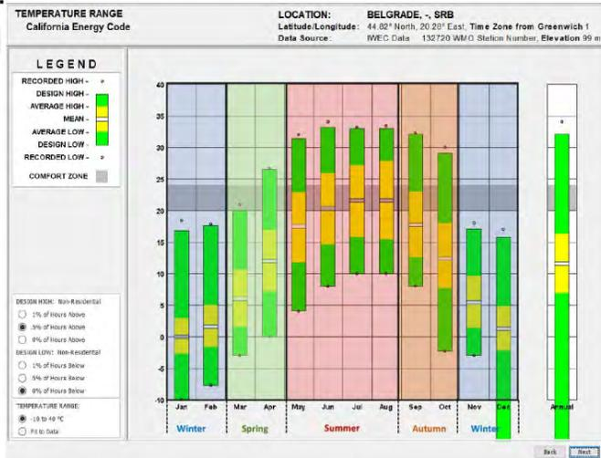
**Graph 1:** The temperature graph shows that in the summer, daytime temperatures get quite high (almost 35 C° on average), but also that during night the temperature drops significantly (almost down to 15 C° on average).
