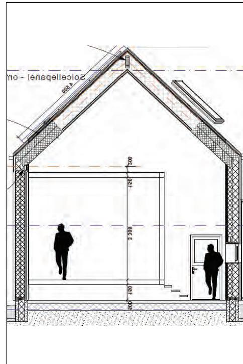
Fig. 2. Section drawing of the ZEB Test Cells
