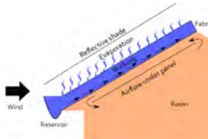
An evaporative cooler (also swamp cooler, desert cooler and wet air cooler) is a device that cools air through the evaporation of water. Evaporative cooling works by employing water's large enthalpy of vaporization.
