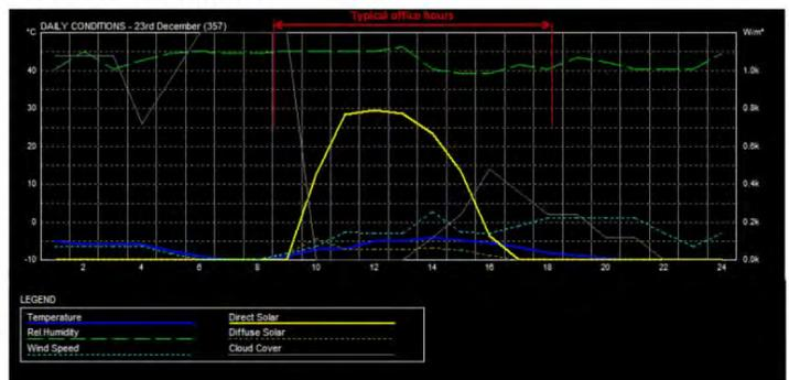
**Graph 2:** Through a confrontation between temperature and direct solar radiation, both in summer and winter, it's possible to observe how there is constant solar radiation during workhours during the whole year.
