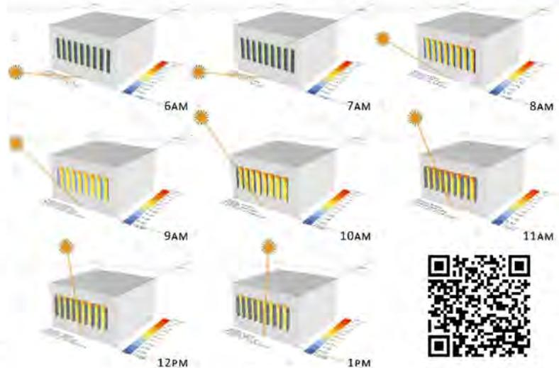
Fig.1: Radiation Analysis, West window | June 21st, 6AM-1PM
