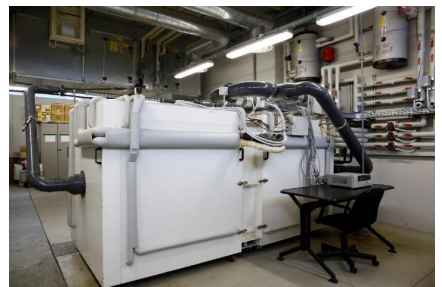
► Fig. 1: Dual Air Vented Thermal Box (DAVTB)
