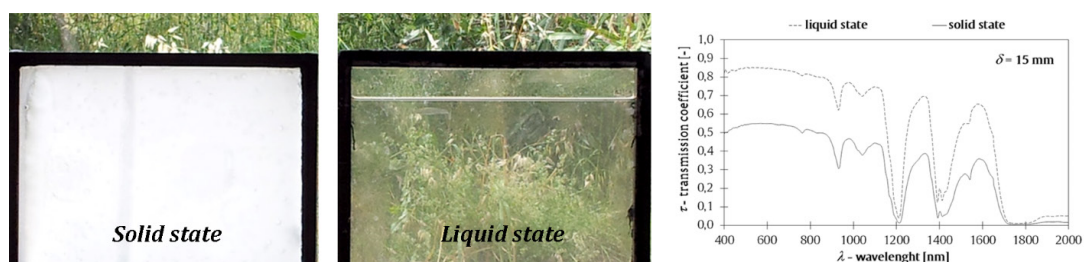
Figure 1 - Appearance of a double glazed unit filled with PCM when in solid state (left) and in liquid state (right), together with the spectral transmittance in the solar range for the two states of aggregation. Source: Goia et al. (2015).
