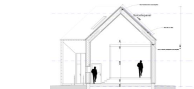
► Fig. 3: Vertical section of the ZEB Test Cells Laboratory with one test cell and one guarded volume.
