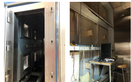
► Fig. 2: View of the two rooms of the Climate Simulator on the left hand side, the cold room with solar simulator, on the right hand the warm room.
