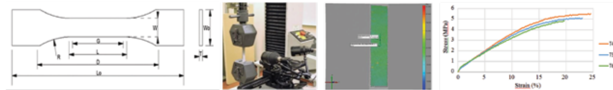
Uniaxial tension tests: Specimen | test apparatus | Aramys stress contours | Results Alexandre Rodrigues et al. (2017)
