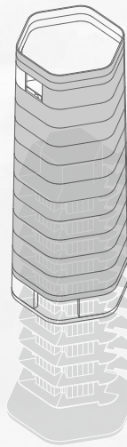
use a loadbearing shell to create an open floorplan and controlled temperatures of ventilation air and moisture levels.
