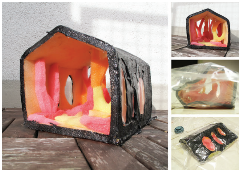
The facade consists of gauze bandage with black latex and is both flexible and completely waterproof. At both sides it will be tied to the foundation, the gauze can handle tensile forces and is thereby holding the house at its place.
