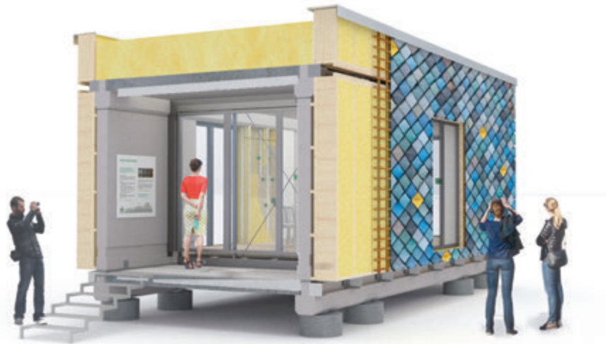
FIG. 2 The Circle House demonstrator is a 1:1 demonstration of circular building systems.
