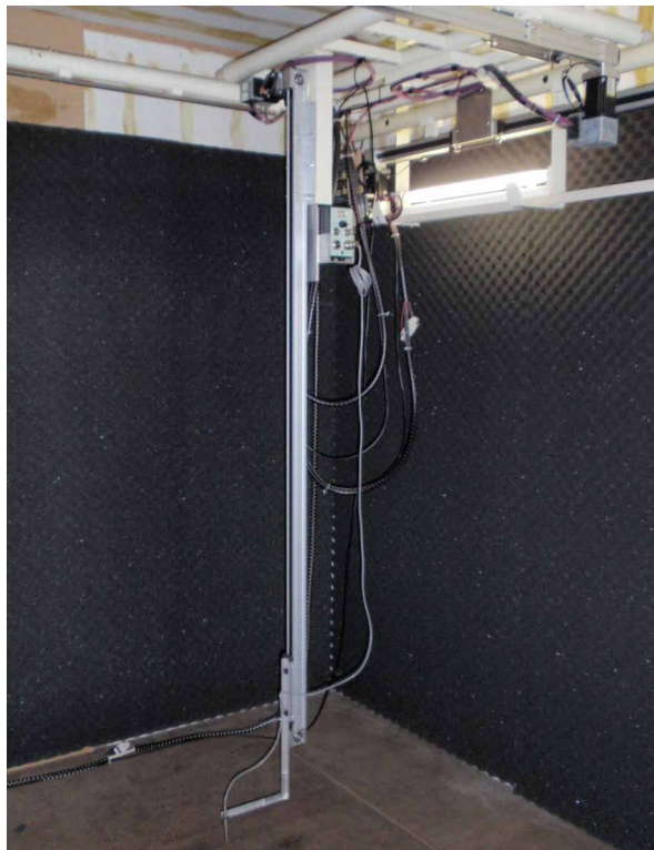
FIGURE 5.1 The 3D microphone positioning rail system at the laboratory at TU Delft, picture by Jelmer Niesten, 2015.
