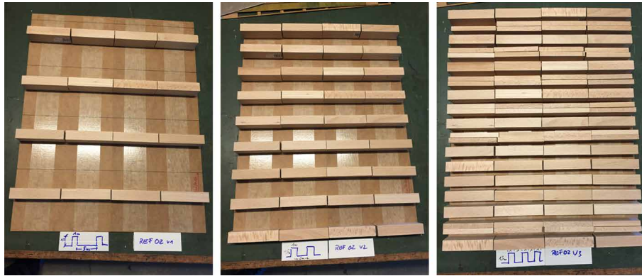
FIGURE 5.7 Horizontal façade geometries comprised of wooden „profile 1“ with three variations for the spacing.
