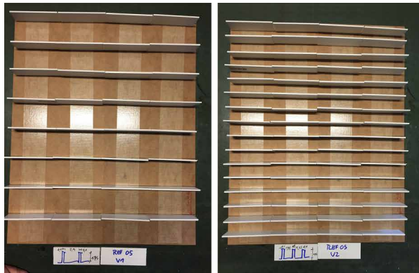
FIGURE 5.8 Horizontal façade geometries comprised of polystyrene „profile 4“ with two variations for the spacing.
