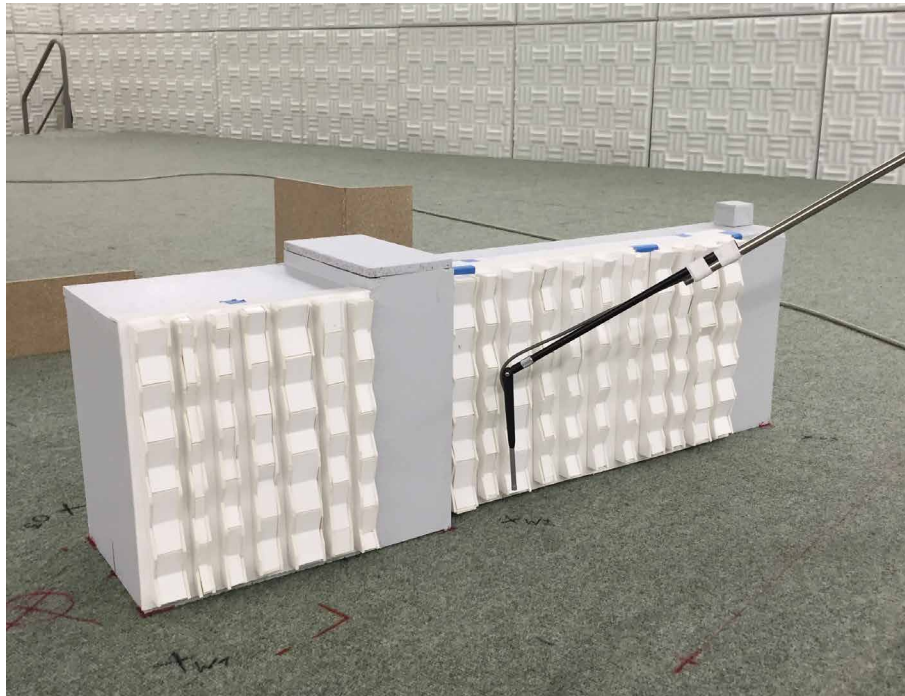
FIGURE 5.34 Model of the building Lyoner Straße 54 in grey colour with the attached façade modification in white measured at position EAST 2. The transparent painted sheets of chipboard in the background represent the façades of buildings in the neighbourhood.
