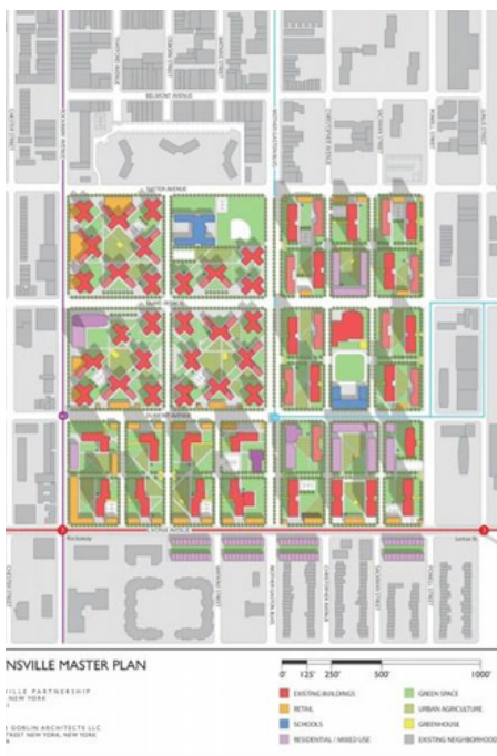
Figure 4: Infill general plan view. Proposal of new affordable-housing(violet) in existing Housing-Project (red) in Brownsville, Brooklyn New York, designed by Alexander Gorlin Office. Commercial areas are proposed (yellow) aligned with new streets. Superblocks can be as big as 4 standard NYC blocks. Source:gorlinarchitects.com
