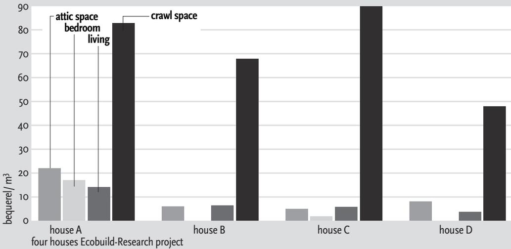
tion may be caused by the ventilation system: house A has natural ventilation, house B heat recovery ventilation.
