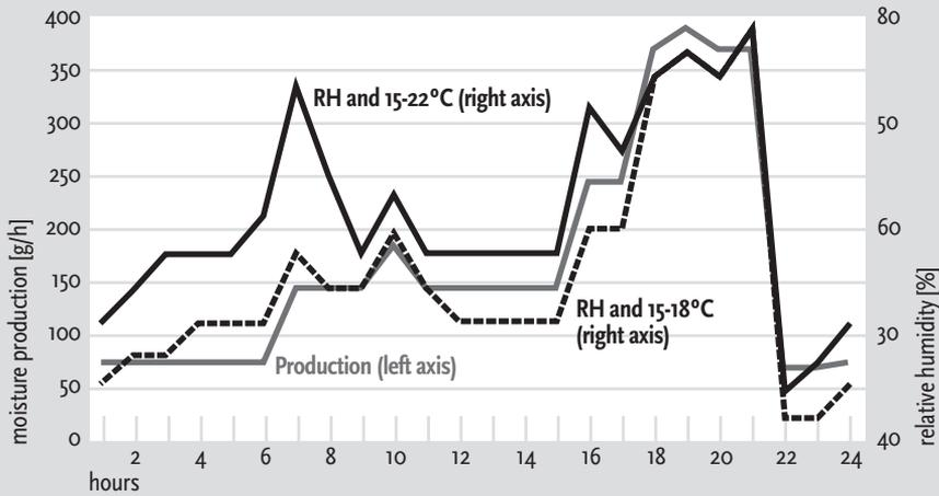
**Figure A3.2** Moisture production and relative humidity RH in the kitchen, ventilation with outdoor and indoor air, calculated on the basis of the moisture production in Figure 4.2 of Subsection 4.3.2
