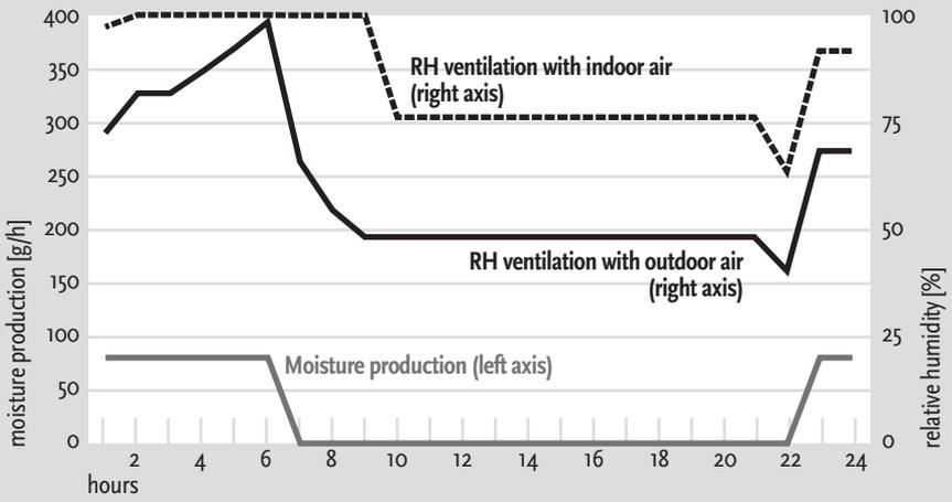
**Figure A3.4** Moisture production and relative humidity RH in the bathroom, ventilation with outdoor and indoor air, calculated on the basis of the moisture production in Figure 4.2 of Subsection 4.3.2
