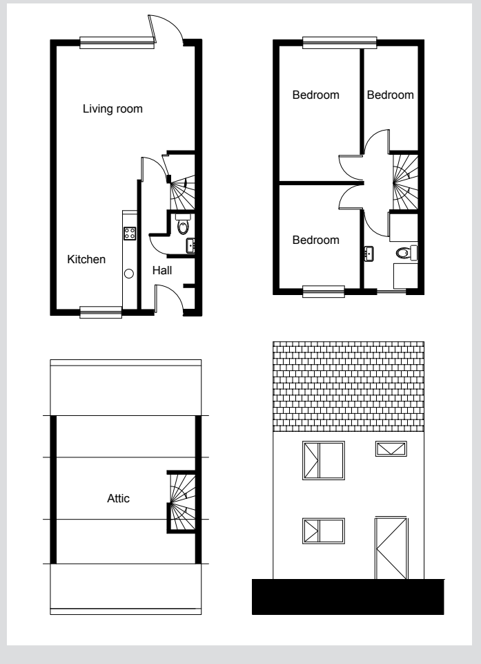
Figure 3.14 Ground floor, first floor, attic and façade of a Dutch reference dwelling
