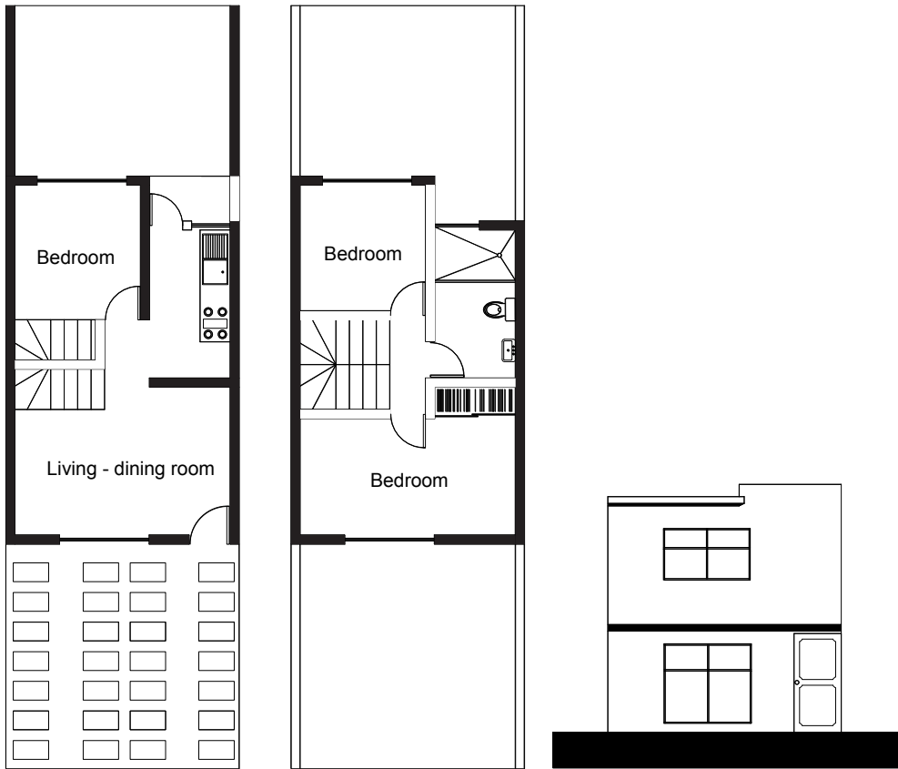
Figure 3.12 Ground floor, first floor and façade of a Mexican social reference dwelling
