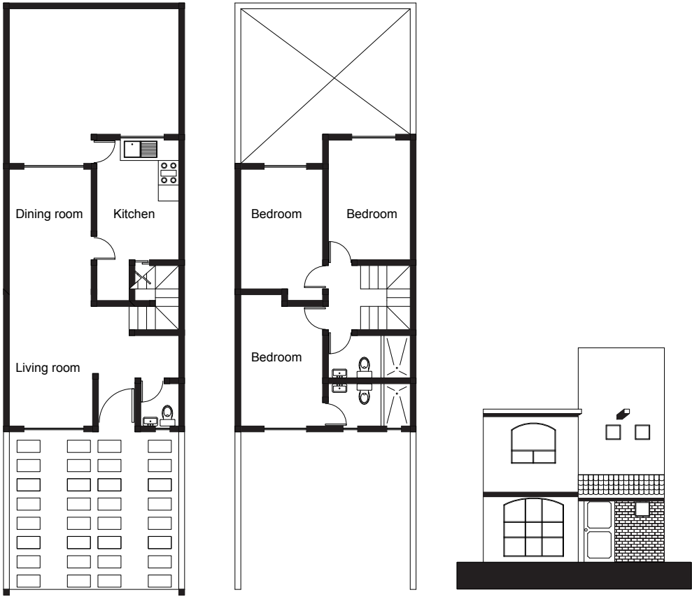
Figure 3.10 Ground floor, first floor and façade of a Mexican medium level reference dwelling
