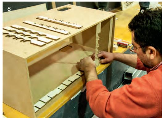
7-8 Assembly of laser-cut results
