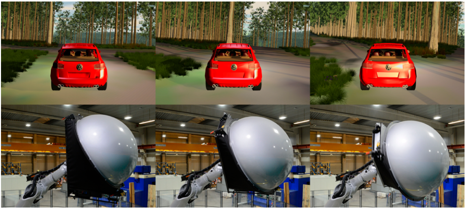
Figure 10. Motion simulator responds to left-hand curve of simulated jeep.
