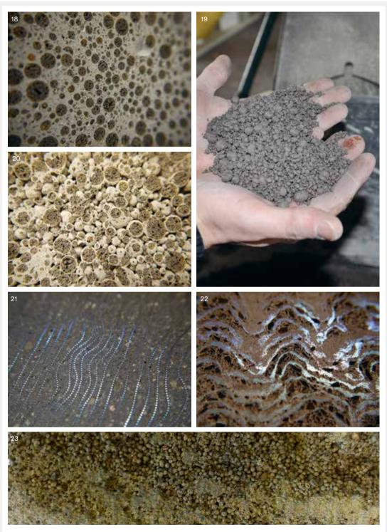
18, 20 Light-weight concrete19 Ultra High performance concrete21, 22 Translucent concrete23 Gradient concrete
