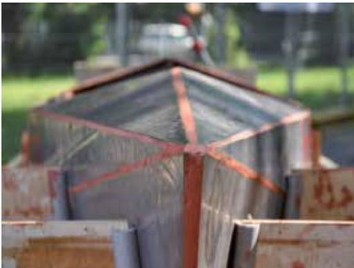
This model and the iterations allowed the team to solve the various problems. The mold of the boat led to different sizes of angles between elements, which meant variable joint spacing. The smaller the angle, the wider the seam distance. The aim was to create a uniform joint, but the new concept did not fit with this aesthetic demand.
