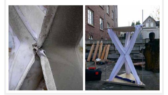
component attached to the short sides of the desk. On the construction side there were many different approaches: the panels were, for example, developed with armoring of textile, glass fiber or steel.
