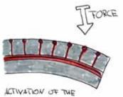
LED'S BY BENDING OF THE CORE LAYERS
