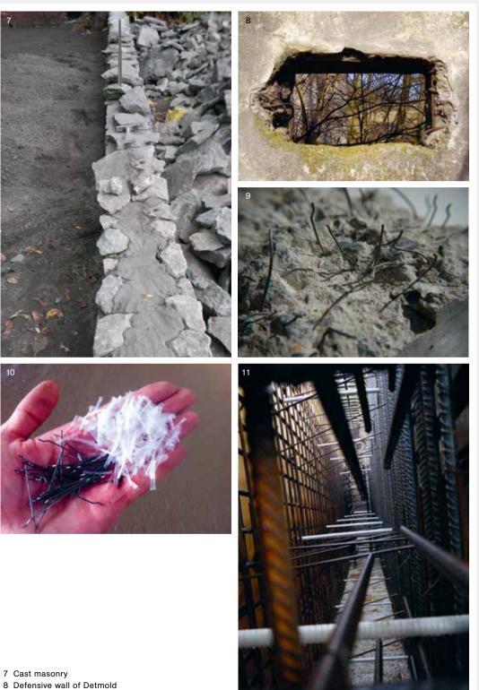
9 Steel fibre concrete
