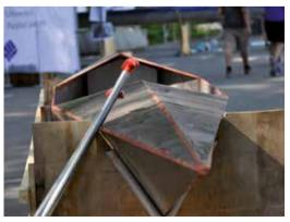
Another group decided to fill up an air mattress with concrete. In order to avoid the air mattress becoming too heavy a light concrete mix was also used. Egg, shampoo and shaving foam were tried as substitute substances, with shaving foam being used in the end. To absorb the pressure at this point, a gypsum formwork was developed. The air mattress was cut open at the upper end to be filled with concrete.
