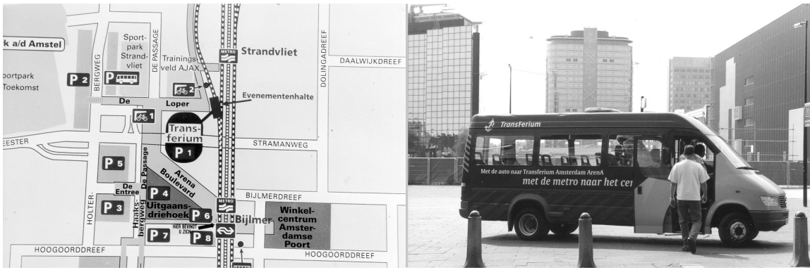
Fig. 4-15 Another example of a poorly designed transport chain, also from Amsterdam South-East, is the situation of the 'transferium' (park-and-ride with public transport connections) near Arena, the Ajax football club stadium. The transferium is sited so far from a metro station that shuttle buses are required between the car parking facility and the metro (the distance between the Bijlmer train and metro station is about 400 metres). Pedestrians are not catered for by directional signs. Not surprisingly, this park-and-ride facility is severely underused. (Photography by the author)
