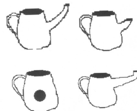
Fig. 5-35 Teapot designs where the law of communicating vessels has been ignored...
