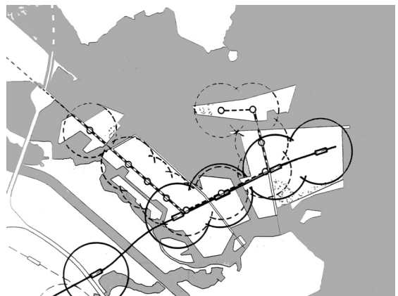
Fig.5-27 Map of the potential accessibility of planned stops on the light-rail system serving an eastward extension of Amsterdam into the IJmeer.
