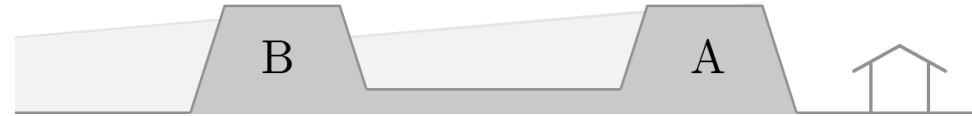
Figure 43. Extreme water levels in case the front defense is not present (either not built or washed away due to failure).
