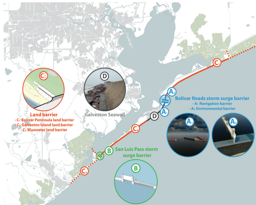
Figure 12. Proposed coastal spine and design elements. (Image Courtesy DEFACTO)
