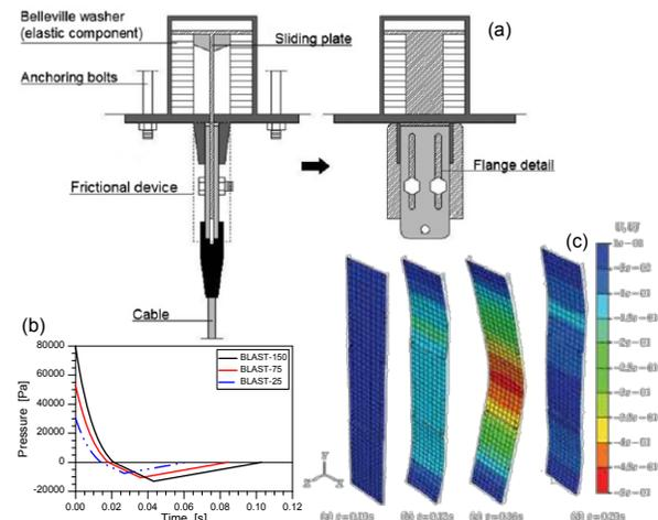
► **Fig. 2:** Example of elasto-plastic passive device for cable-net façades [4]. (a) Schematic view; (b) air blast time-pressure wave; (c) dynamic response of a cable-net modular unit (University of Trieste, Italy).
