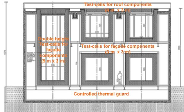
► Fig. 1: Front view of design plans for the Tipee's test cell facility drawn by architect team AIA
