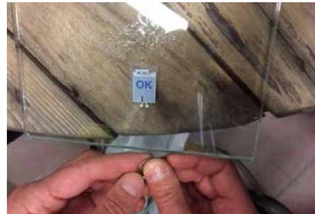
▶ Fig. 2: An example of how printed electronics can be integrated in glass. Here, a printed display has been added to a laminated glass light.
