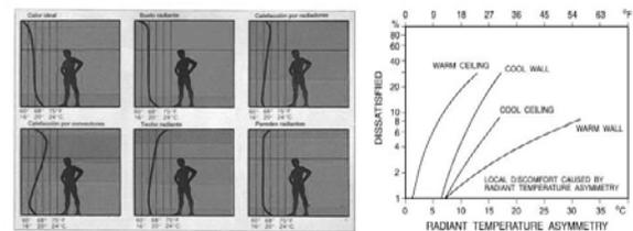
Fig. 3: Gradient of the temperatures for different types of heating systems; and diagram of Predicted Percentage of Dissatisfied (PPD) for radiant temperature asymmetry by different heating systems, according to ASHRAE 2001.
