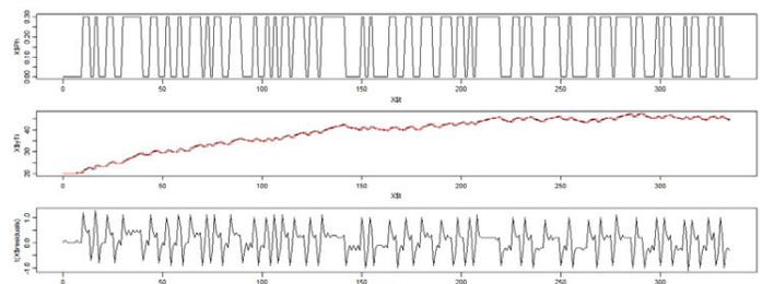
► Fig. 3: Typical heating impulse sequence, indoor air temperature measured (black) and fitted (red), residual function of an identification process (model TiTeTh, Bermanni's Master Thesis)
