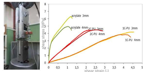
► **Fig. 3:** Testing of adhesive connection; influence of adhesive layer on
