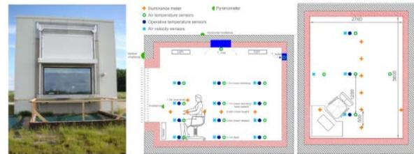
▶ Fig. 1: Full-scale test facility in Aalborg University - Cube. (Left: test facility, Right: section with measurement points).
