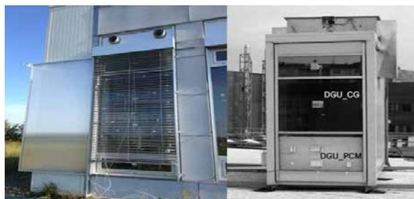
► Fig. 2: Experimental setup with external insulation shutter and venetian blind (left), experiment of glazing integrated with PCM (right).
