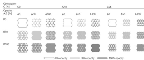
► **Fig. 2:** Twenty-seven configurations of shadings: no shadings (A0; B0), complete shading (A100; B100) and mixed combinations of opacity for the A and B faces, each for a specific rate of contraction.
