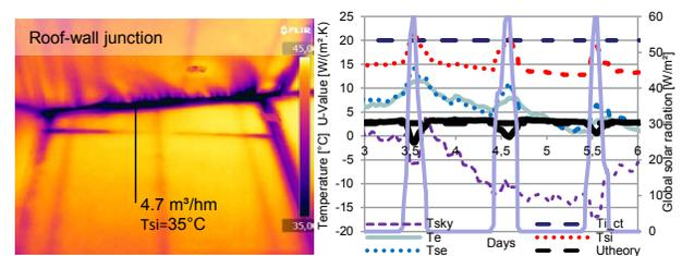
► **Fig. 3:** Left: IRT visualization of air flow rates inside a test house. Right: DGU with argon filling, simulated with reference weather: Comparison of theoretical and simulated U-value. The accuracy of U-value estimation with IRT improves when avoiding solar radiation and a clear sky.
