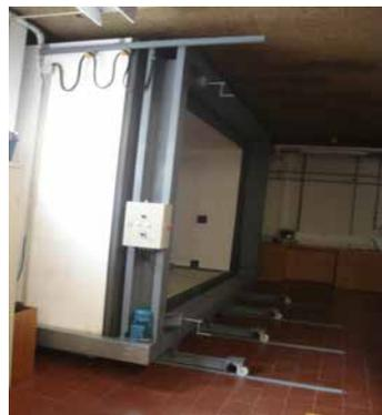
► Fig. 2: Thermal and acoustic chamber and outdoor test cell
