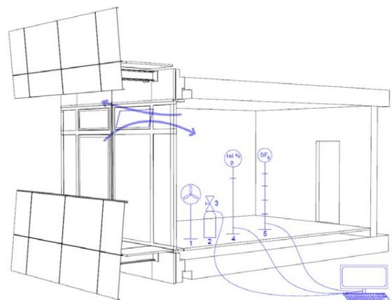
► Fig. 2: Façade test laboratory with tracer gas equipment
