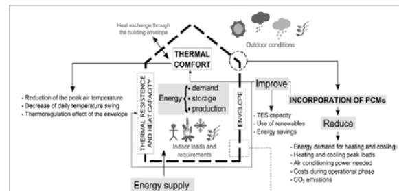
► Fig. 3: Sketch of the building as a thermodynamic system and main advantages of incorporating TES systems with PCMs in buildings.
