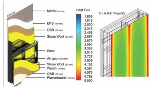
► Fig. 1: Thermal performance of a LSF wall: heat flux.
