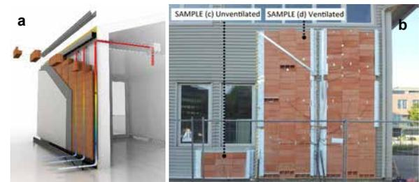
▶ Fig. 4: a) Ventilation scheme of the supply air configuration, b) Outdoor test in laboratory building of POLITO.
