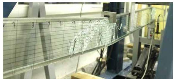
► **Fig. 2:** Structural glass research: robustness of reinforced hyperstatic glass members, including safety after accidental removal of intermediate support.
