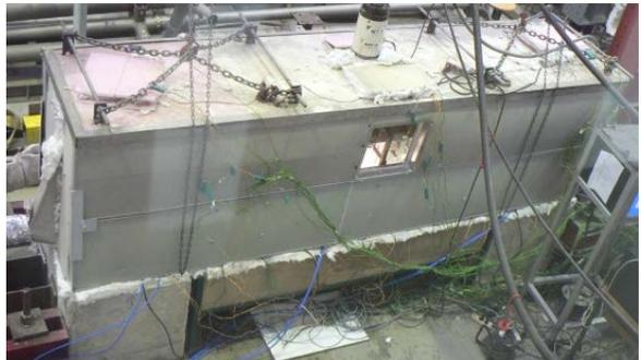
► Fig. 3: Thermal conditioning chamber for glass testing, University of Coimbra
