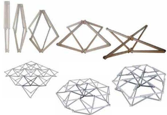
► **Fig. 1:** Kinematic systems: uneven Sarrus chains. Top: basic module; Bottom: i) Flat rectangular joint-to-joint array, ii) Flat hexa-triangular joint-to-joint array, iii) Flat hexa-triangular overlap array
