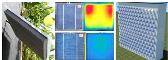
► Fig. 3: Bionic leaf (left) enhancing electricity production (centre), evaporative cooling and shading of the building envelope. Bionic leaf is a basic structural element of the bionic façade (right), mimicking VGS.
