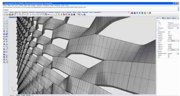
► Fig. 3: Grasshopper interface for the expanded metal 3D modeller and example of resulting model
