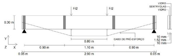
► Fig. 1: Layout for the full scale tests as part of the S-Glass project at the University of Coimbra (pre-stressed non-hybrid system)
