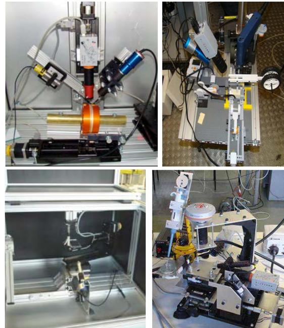
▶ Fig. 3: Experimental set-up for multi-scale characterization of bio-based materials performance
