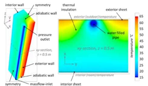
▶ Fig. 2: Three-dimensional thermal reference CFD model (RF) and a section through the xy-surface with temperature contours at the middle of the panel’s height (z-length = 0.5 m) for summer conditions.
