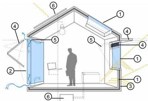
► **Fig. 2:** Adaptive building components energy and comfort simulation capability of the tool/method developed within the gFT: 1. Construction properties; 2. Surface heat transfer; 3. Material surface properties; 4. Schedules; 5. Openings; 6. RES generation and storage.
