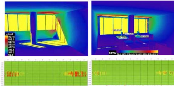
**Fig. 1:** Behaviour analysis of shading system of the basic unit of an office building (numerical and graphical daylight simulations)
