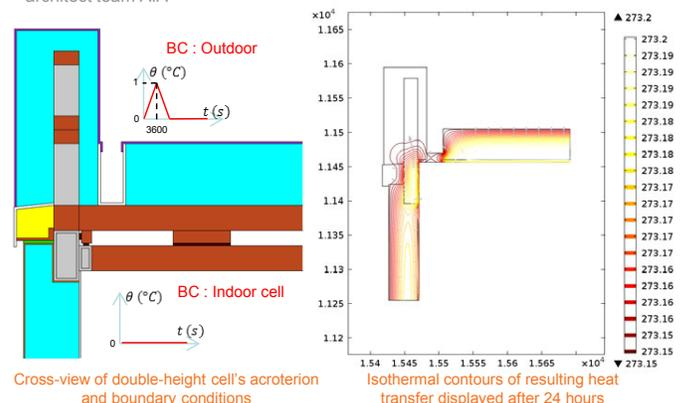
► Fig. 2: Evaluation of linear thermal bridge in a time-dependent heat transfer
