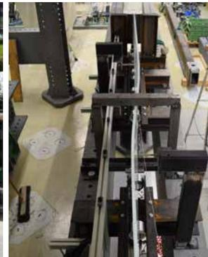
▶ Fig. 2: Double waved buckling on glass beam during a test
