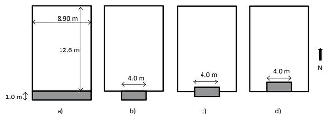
► Fig. 2: Building floor dimensions and sunspace configurations
