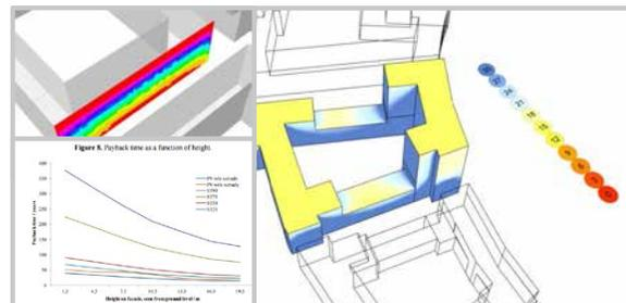
► **Fig. 1:** Assessment of integration profitability of solar systems in the urban built environment: e.g. the solar facade tool FASSADES shows the profitability of solar surfaces vs payback time. (J. Kanters)
