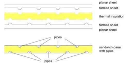
▶ Fig. 1: Solar activated sandwich panel (cross section).
