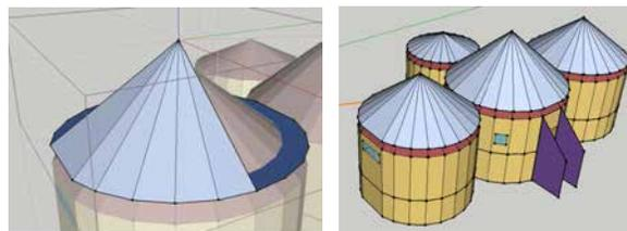
► **Fig. 1:** Numerical simulation for energy optimization of an experimental construction. Influence of weather conditions, materials, roof shading, window size, glazing, cross-ventilation, etc.
