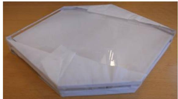
▶ **Fig. 3:** New type of a cross flow energy exchanger using membrane technology developed at the Research Centre
