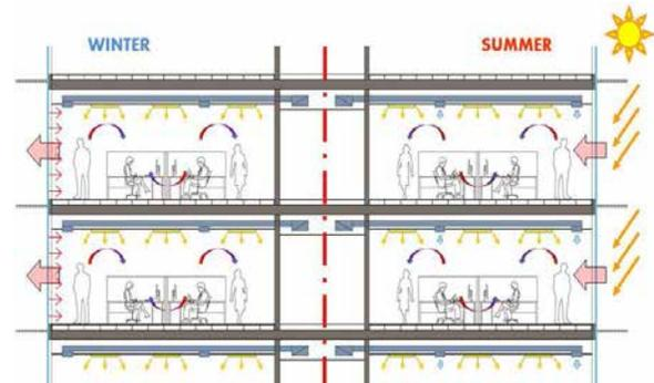
Fig. 1: The heating exchange between the environment and the office building through a glass envelope equipped with Radiant Glass Façade, during summer and winter.
