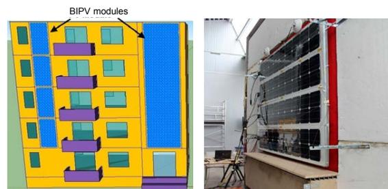
a. Dynamic simulation of building integrated photovoltaics with TRNSYS
