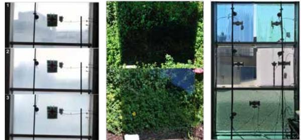
▶ Fig. 3: Prototypes tested (thermotropic, thermochromic and polycarbonate filled with PCMs).
