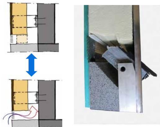
► **Fig. 2:** Basic principle and actual implementation of an opaque switchable insulation with convection control in a back-venting gap. In order to prevent heat bridges at the openings of the gap, the doors are insulated with a high-performance, aerogel based insulation material. The main insulation in the example element is a standard PU foam
