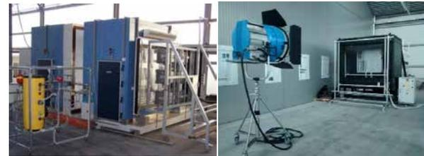
a. INTENT guarded hot-box double chamber, sun simulator, hydraulic circuit
