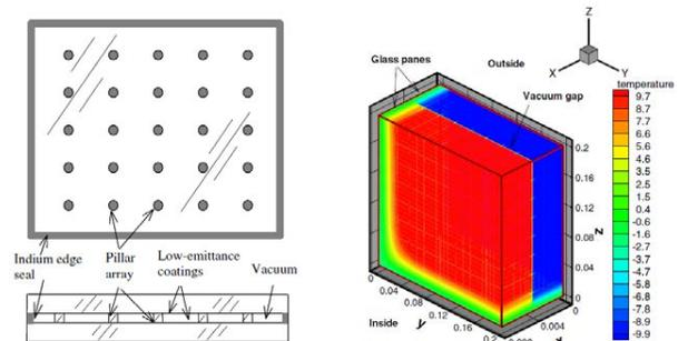
► **Fig. 1:** Left: Schematic diagram of a vacuum glazing. Right: Predicted isotherms for a vacuum glazing with coatings of emittance 0.12 and 0.16 on the two glass pane surfaces within the vacuum gap.
