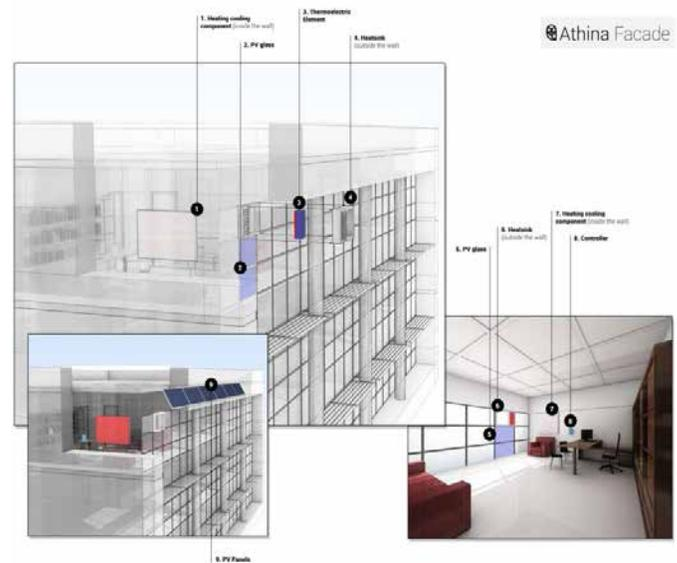
► Fig. 1: The ATHINA components: Heating-cooling component, PV glass, thermoelectric element, heat sink
