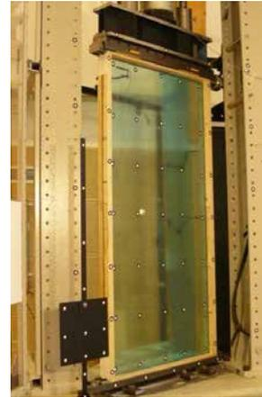
▶ Fig. 1: A glass/timber shear wall element being tested at Linnaeus University in Växjö, Sweden.
