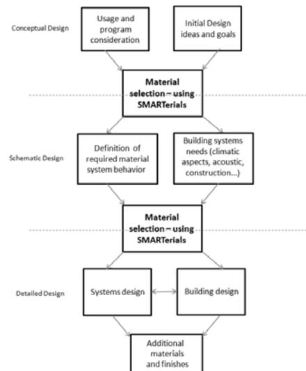
► Fig. 1: Flow chart of the design process integrating the SMARTerials tool.
