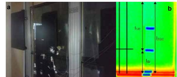
▶ Fig. 5: a) The glazing unit equipped with sensors inside the BET cell apparatus, b) Thermal bridge infrared image.
