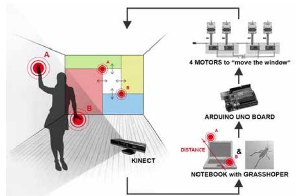
Fig. 2: IFDC efnMobile Workshops Lucerne 2014: Movable window using Kinect and Arduino UNO to detect the movement of the hand to control the Movable Window.
