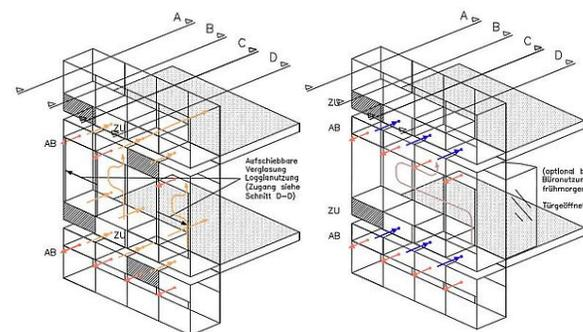
► Fig. 3: Variable air flow directions in climatic case III (left) and IV (right)
