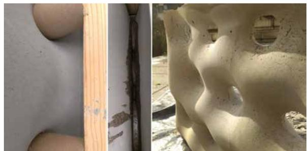
► Fig. 4: Experiments with latex formwork / Sasha Hickert
