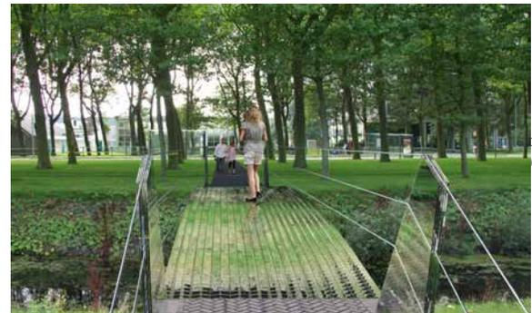
▶ Fig. 2: Rendering of a dry assembled glass brick bridge design (rendering by XKP visual engineers)
