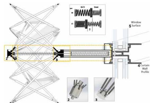
► Fig. 2: Section of the shading component: 1. SMA smart thermal actuator that works against the bias compression spring to create linear motion. 2. 3D printed spherical joint 3. 3D printed spherical joint with a connector for a metal tube. 4. The connection to the curtain wall profile.
