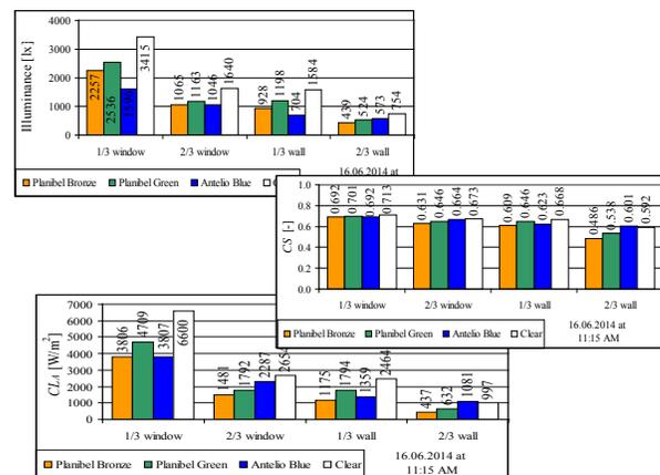
Fig. 4: Photopic illuminance levels recorded at all positions in all models - CLA levels estimated with Rea's equation for all positions in all of the models - Computed CS levels acquired from Rea's model in all positions in all of the models
