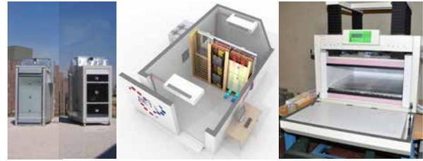
▶ Fig. 1: Outdoor test cell units (TWINS), Building envelope test cell (BET cell), Guarded Heat Flow Meter (GHFM)
