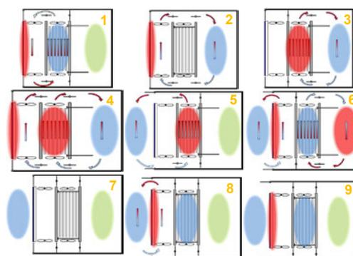
Fig. 4: Different operation modes of BIPV/T-PCM system. Green is the indoor zone, blue is cold air and red hot air. Operations modes from 1 to 4 and 7 are for heating season and 5, 6, 8 and 9 are for cooling season.
