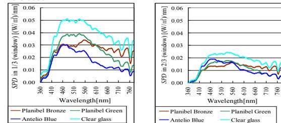
Fig. 3: SPD levels recorded in 1/3 and 2/3 of the model room's length – sensor oriented toward window
