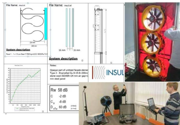
► Fig. 2: The influence of new materials and solutions on facade airborne sound insulation is predicted by calculation and checked by testing of large-scale models or in completed buildings. “Blower door” tests also show the performance of new solutions.
