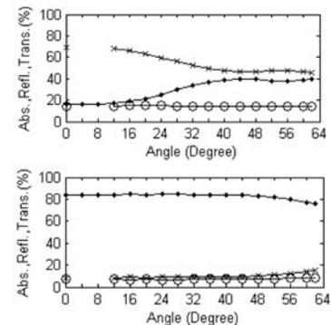
► **Fig. 2:** Average transmission (dots), reflection (crosses) and absorption (circles) of a chiral liquid crystal switchable mirror in the 380-780nm range with light incidence angle in the reflective state (top) and clear state (bottom).
