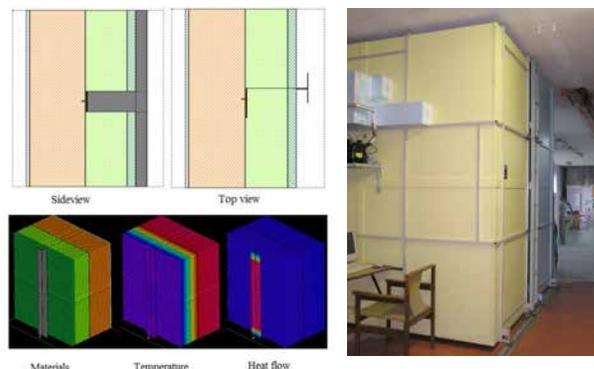
► Fig. 1: For the introduction of new elements into the facade network, we provide 3D calculation and determine the U-value of facade fragments in a “Hot Box”
