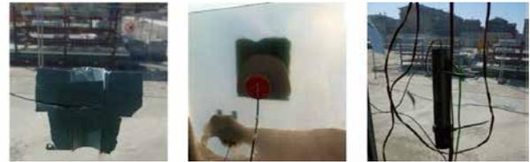
▶ Fig. 2: Shielded sensors and ventilated thermocouple for energy performance measurements of advanced transparent building components
