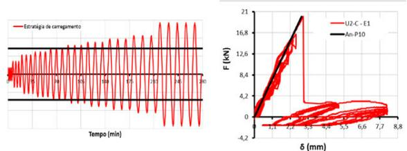
► Fig. 3: Cyclic tests: Load strategy and damage in elastic and post fracture regimen.
