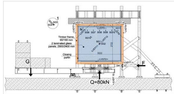
► Racking test set-up and instrumentation of specimen
