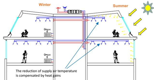
► Fig. 1: The reduction of supply air temperature is compensated by heat gains
