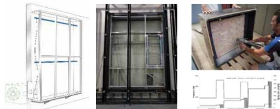
► **Fig. 4:** Water tightness test: both rain and wind are simulated. Wind effects are represented by pressure differences generated by a fan (green). Rain is provided by means of water spraying nozzles in front of the test setup (blue).
