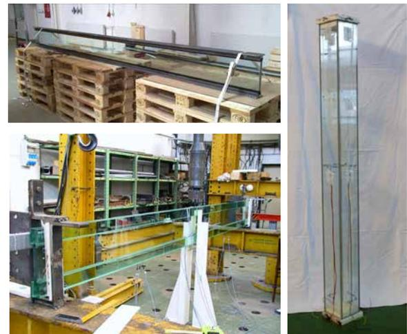
► **Fig. 2:** Structural elements with essential usage of adhesive joint,
