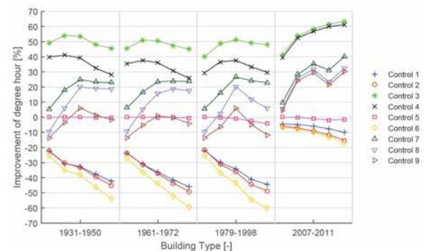
▶ Fig. 2: Potential of using dynamic facades with different control strategies related to the indoor thermal climate.
