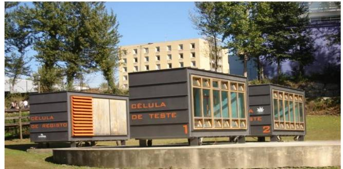
► Fig. 1: Real scale test cells
