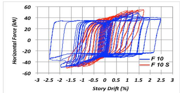
► **Fig. 3:** Response diagrams of original and repaired double-glazed frame with φ14mm rod test setup and instrumentation of sample
