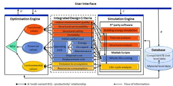
► **Fig. 1:** Multi-objective assessment and optimisation tool for façades developed within the gFT research group. This SW framework is the basis for different ongoing research projects within the research group.
