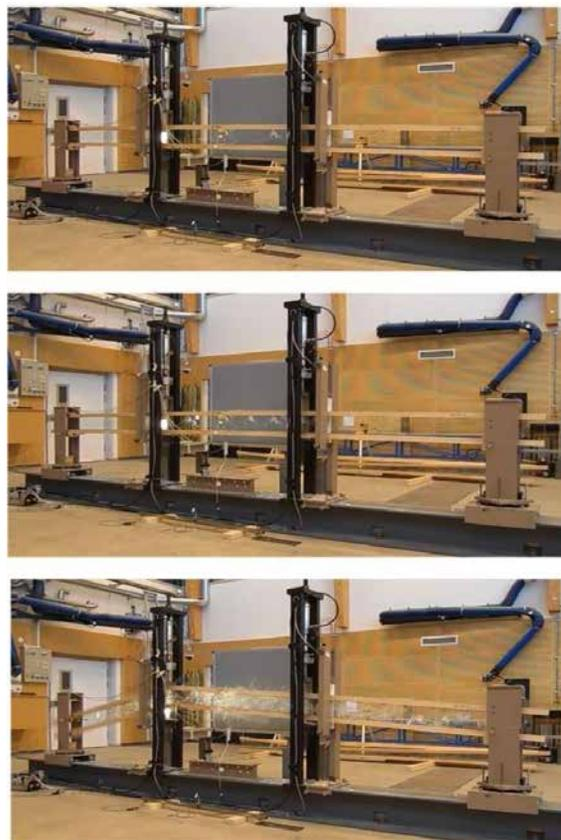
► **Fig. 1:** Progressive damage of timber-glass beam with annealed float glass
