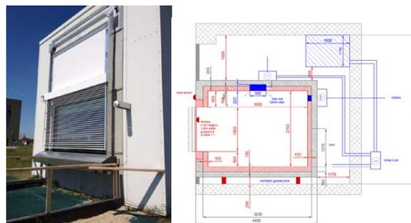
► Fig. 1: Full-scale test facility in Aalborg University, the Cube. (Left: test facility, Right: section).
