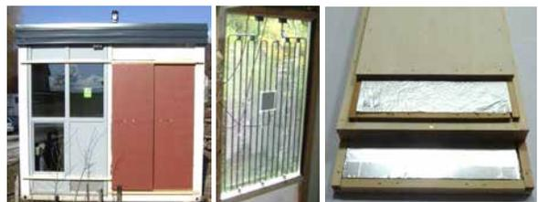
► Fig. 4: Outdoor laboratory site (left), where adaptive façade technologies, such as glazed SC absorber (centre) and lightweight panel with VIP and PCM layer (right), are tested.
