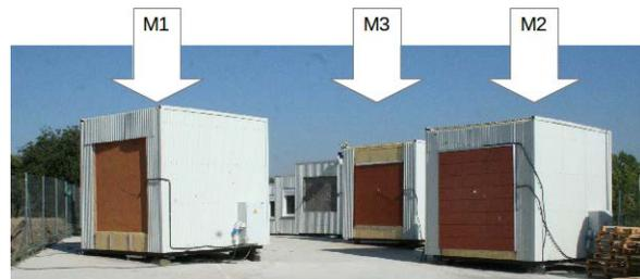
▶ Fig. 3: Tested systems for facade refurbishment (REFAVIV project)
