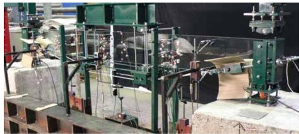
► Fig. 2: Experimental setup for the full scale tests as part of the S-Glass project at the University of Coimbra (pre-stressed non-hybrid system)
