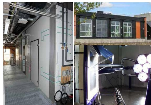
► **Fig. 3:** EBD test facilities for façade systems - outdoor façade laboratory (left and upper right) and solar energy technologies - indoor full-scale solar simulator (lower right)
