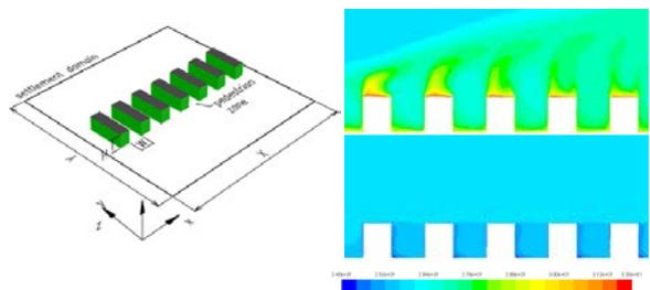
► Fig. 2: Evaluation of urban heat island mitigation potential using combined TRNSYS – CFD model. Comparison of UHI of the grey urban canyon (right top) and engaging VGS (right bottom).
