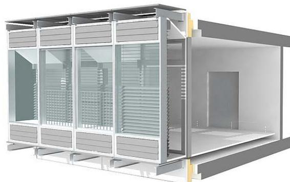
► Fig. 1: Rendering of the test room equipped with a bypass double skin facade
