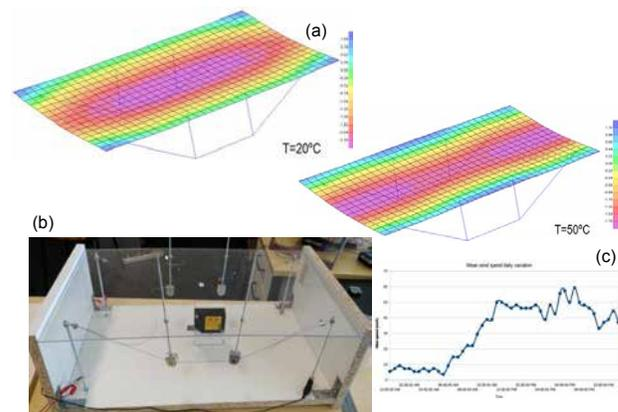
► **Fig. 3:** Adaptive glass panel, with smart cable system. (a) Finite element simulations; (b) smart panel prototype and (c) wind pressure daily variation (Universidade Nova de Lisboa, PT)
