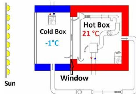
▶ Fig. 3: Small Hot Box system with artificial sun (OSRAM Ultra-Vitalux)
