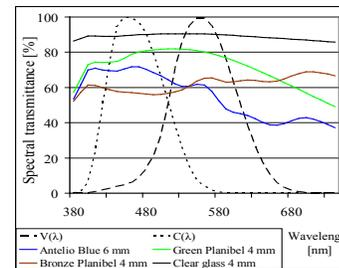
Fig. 2: Spectral transmittances of the tested glazing plotted over the sensitivity curves of circadian and visual systems. Types: Planibel Bronze 4 mm; Planibel Green 4 mm; Antello Blue 6 mm and clear glass 4 mm were used.
