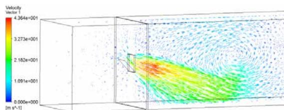
► Fig. 3: Exemplary numerical simulation of the airflow through a bottom pivoted window
