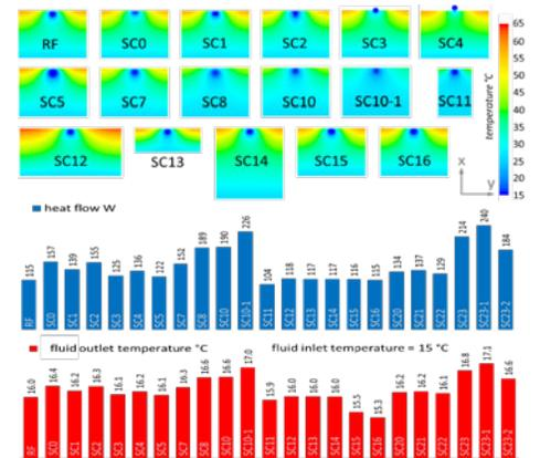
▶ Fig. 3: Comparison of the temperature contours & of the non-area-weighted heat flow of a single pipe and the fluid outlet temperature between the RF scenario and the scenarios SC0 - SC16.
