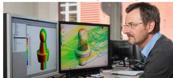
▶ Fig. 3: CFD wind simulation of a radar station on a summit
