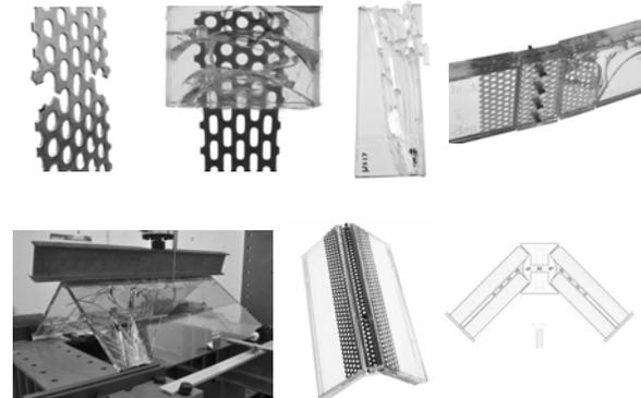
► **Fig. 2:** Different tested specimens used during the experimental investigation.
