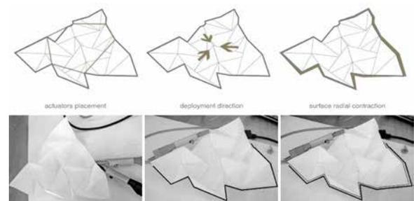
► **Fig. 3:** The actuators placement allows envisioning the deployment direction. To prevent local deformation, the experiment did not take into account connection wires from the boundary vertexes to the central vertex.
