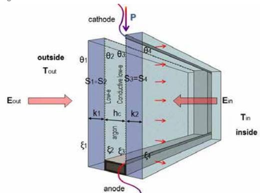
Fig. 2: Diagram of a Radiant Glass Façade, and variables used to determine the thermal balance.
