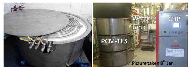
► **Fig. 3:** Left: PCM-TES storage unit prototypes (0.52m tall by 1.45m diameter) developed to TRL7. Right: Three PCM-TES units stacked in a test bed laboratory fired by a CHP unit
