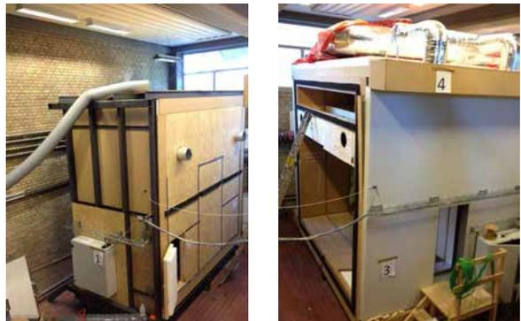
▶ Fig. 2: Large Hot Box system. Cold zone (left), hot zone (right)
