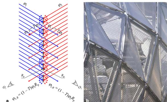
► **Fig. 3a:** Section through the perforated plate. Initial luminous fluxes are marked  $\phi_1$  and  $\phi_2$ .  $O_1$  and  $O_2$  are the observers of the scene. **Fig. 3b:** The perforated metal shell is like cellular polycarbonate. The Island on the Mur in Graz, AT (arch. Vito Acconci).
