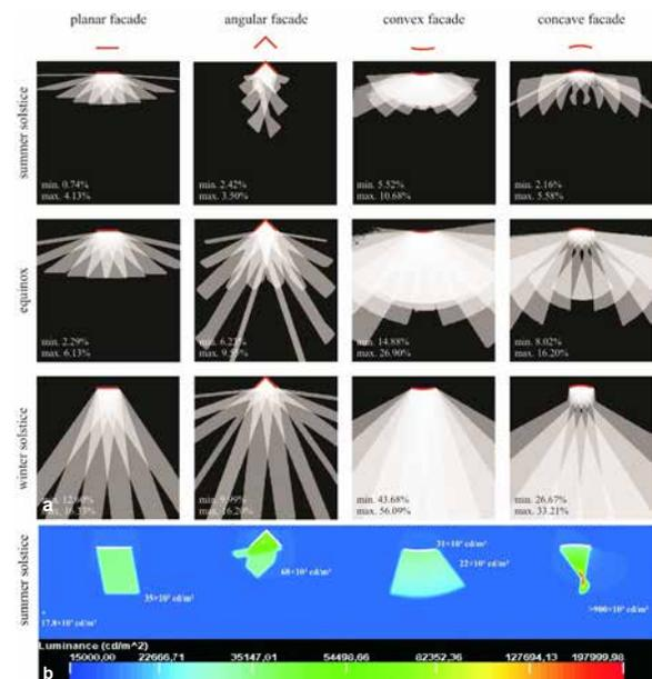
► **Fig. 2a:** The glare reflected off the smooth façade on the ground for south-facing test façade at different times of the year for different façade shapes. **Fig. 2b:** Façade glare intensity in false colour.
