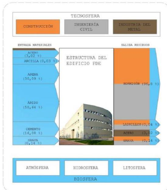
► **Fig. 3:** Material Flow Analysis methodology applied to a building of the Cappont Campus at the University of Lleida. The methodology aims at reducing and managing the materials and waste produced at the end of the life span of the building
