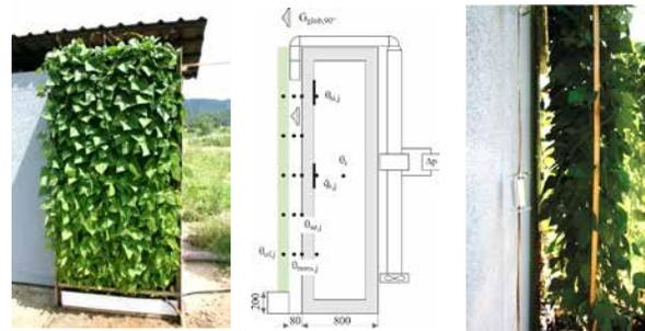
► Fig. 1: Experimental setup for evaluation of thermal response of vertical greenery systems (VGS).
