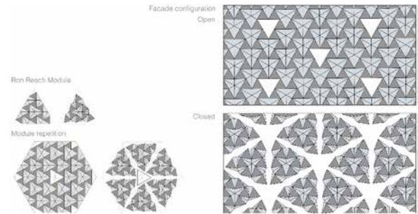
► **Fig. 1:** Ron Resch pattern module geometry allows to repeat the pattern on different scales, creating a self-similar pattern. The repetition of hexagonal modules gives an example of facade's integration.
