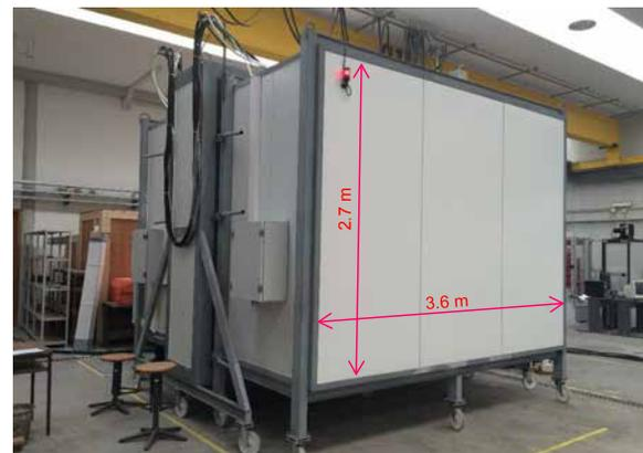
► Fig. 4: Guarded Hot Box Test Station developed at University of Coimbra.
