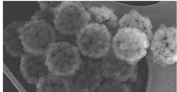
▶ **Fig. 1:** Microscopy of a Nano Insulation Material (NIM) developed at the Research Centre
