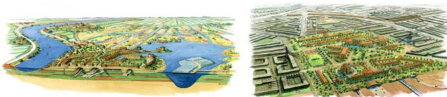
Figure 13 New neighbourhoods on mega-mounds to avoid an increase in flood damage and thus flood risk (designed by landscape architects Stroming. Images taken from: Aerts et al. 2008)
