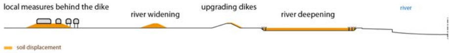
Figure 1 Three ways to reduce flood risk, next to disaster management and measures to redirect flows on a higher scale level (like a storm surge barrier or a spillway near a river bifurcation)
