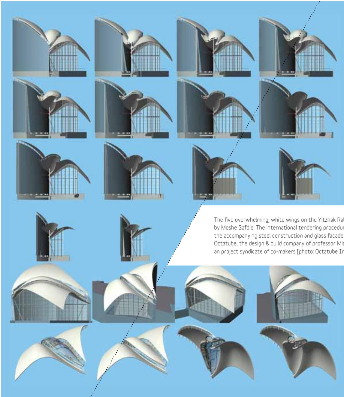
The five overwhelming, white wings on the Yitzhak Rabin Center in Tel Aviv by Moshe Safdie. The international tendering procedure for the roofs with the accompanying steel construction and glass facades was won in 2005 by Octatube, the design & build company of professor Mick Eekhout PhD, and an project syndicate of co-makers [photo: Octatube International].
