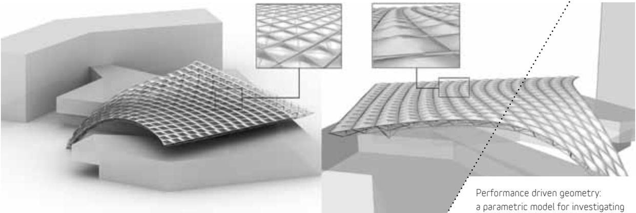
Performance driven geometry: a parametric model for investigating alternative configurations of the cladding for reducing direct solar exposure (by Michela Turrin et al).
