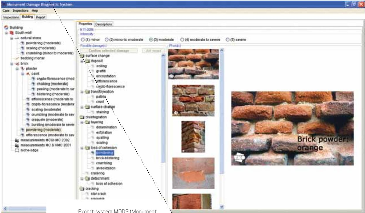
Expert system MDDS (Monument Damage Diagnostic System) - Screenprint of an analysis of brick decay.
