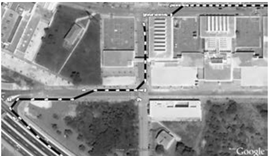
Illustration 12.3 Filter application to a GPS trace. The arrows indicate trace points, while the thick line corresponds to the filtered path proposed
